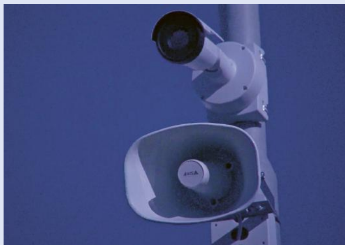
Network speakers are a speciality within Axis' product portfolio and have also become increasingly common in perimeter security applications.
