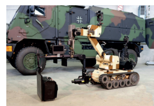
Battery operated X-ray tubes and digital detectors create a high-resolution image that highlights even smallest wires and igniters.
